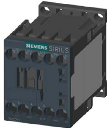
CONTACTOR, AC-3, 3KW/400V, 1NO, AC 24V, 50/60 HZ, 3-POLE, SZ S00 SCREW TERMINAL
